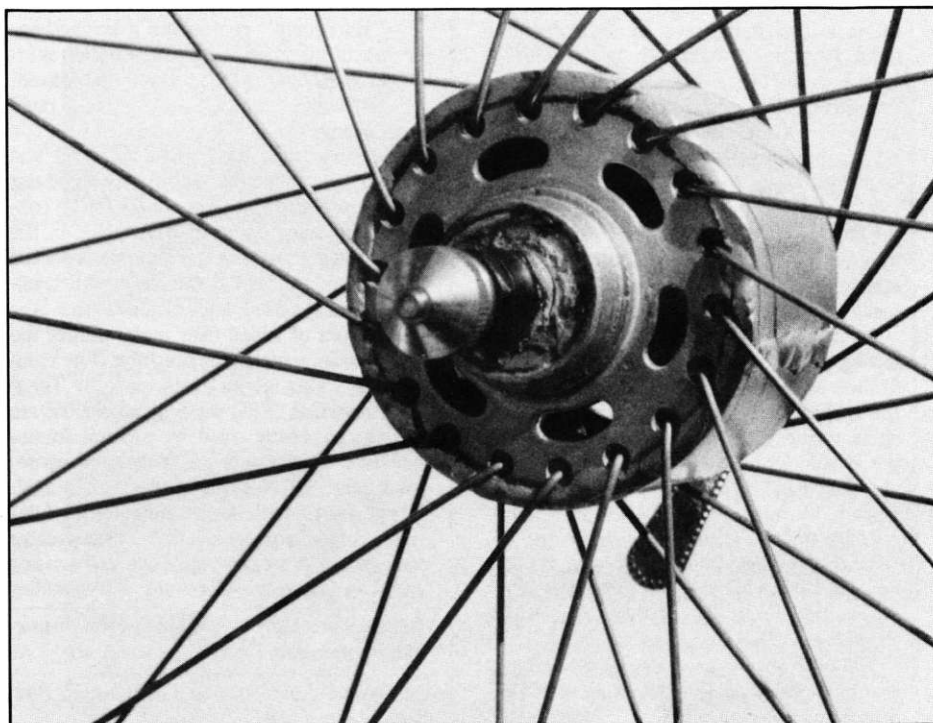
A left-all-pulling, right-all-static wheel built around a special rear hub strengthened to resist the twist of one flange relative to the other. [Reprinted with permission.]
